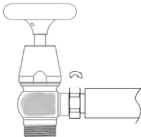
4. Insert the pipe (at this point you will have already prepared the water supply pipes to match up with the radiator or towel rail and valve dimensions). Then tighten the nut (with the olive already in place) that holds the pipe in position.
